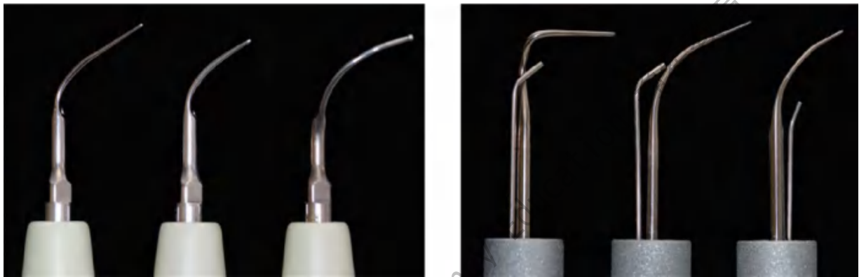
Fig. 30-8 Inserts of different length and curvature for piezoelectric (left) and magnetostrictive (right) ultrasonic devices.
